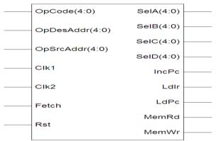
Fig.11: Block Diagram of Control unit
