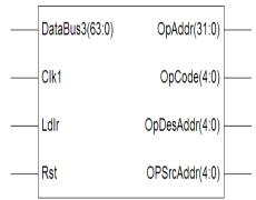
Fig.2: Block Diagram of Instruction Register
