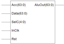
Fig.5. Block diagram of ALU
