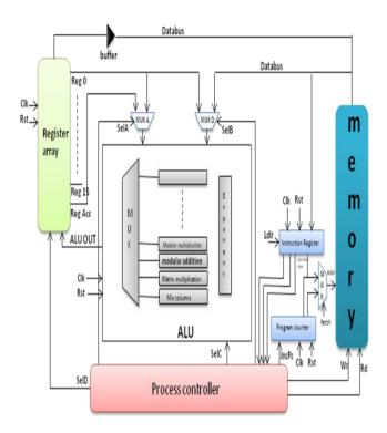
Fig.1: Processor Architecture
